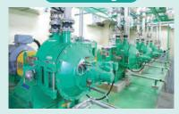
To ensure a strong paper with well-combined fibers, the fibers are then thoroughly ground so that they combine easily.
