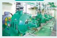
To ensure a strong paper with well-combined fibers, the fibers are then thoroughly ground so that they combine easily.
