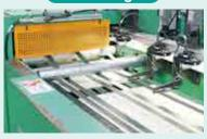
The rolled paper is cut into sheets of the right size for printing and sent to the next process of printing.
